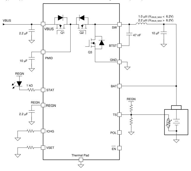
Figure 9-1. Typical Application Diagram
