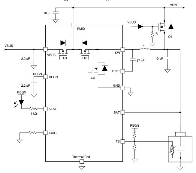
Figure 9-7. Typical Application Diagram with Power Path
