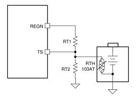
Figure 8-3. Battery Temperature Sensing Circuit
