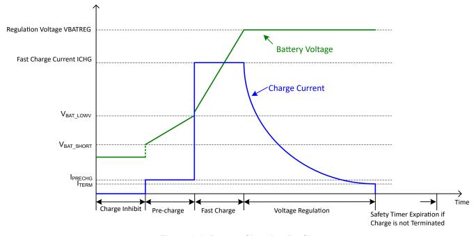
Figure 8-1. Battery Charging Profile
