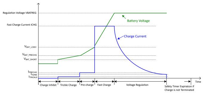
Figure 8-2. Battery Charging Profile for V<sub>BATREG</sub> = 3.6V
