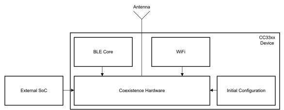
Figure 6-1. Coexistence in CC33xx Device
